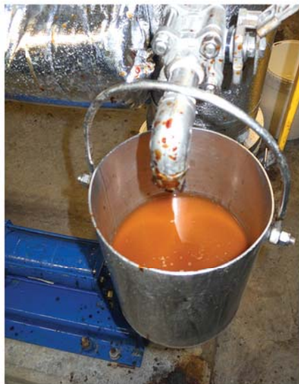
A pail of Pot Ale Syrup an animal protein supplement, the product from pot ale processing facility. Using steam and power from the CHP it can turn 430 000 tonnes pot ale into 44 000 tonnes "Spey Syrup" per year. It doesn't taste half bad either.
